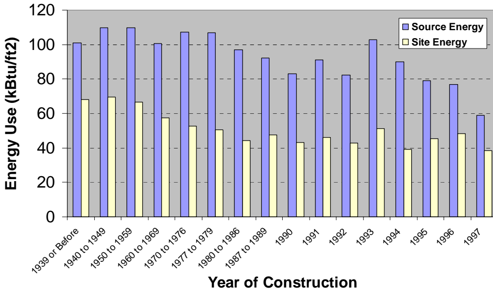
Figure 9. Normalized site and source energy consumption by year of construction (EIA, 1999), illustrating downward trend for more recent vintages. Note: Source energy includes generation and distribution losses for electricity.
